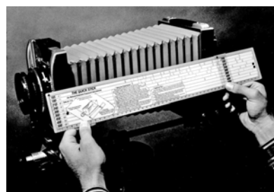
The Quick Stick for bellows extension exposure calculations on large format cameras
